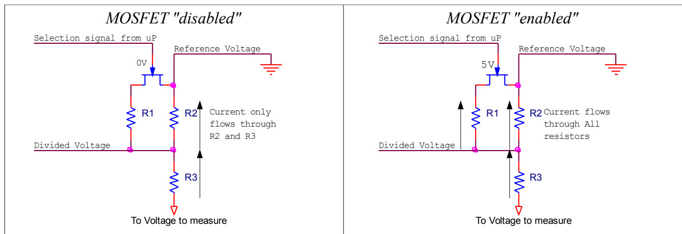
Figure 9: Selectable High Impedance Voltage Divider
